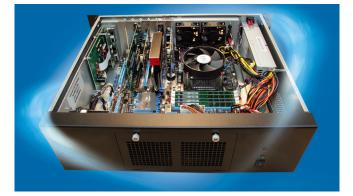
The new arrangement of the fans in the HEITEC chassis enables smart heat management
