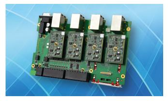
PCB of the unit with a view of the four interchangeable interface boards.
