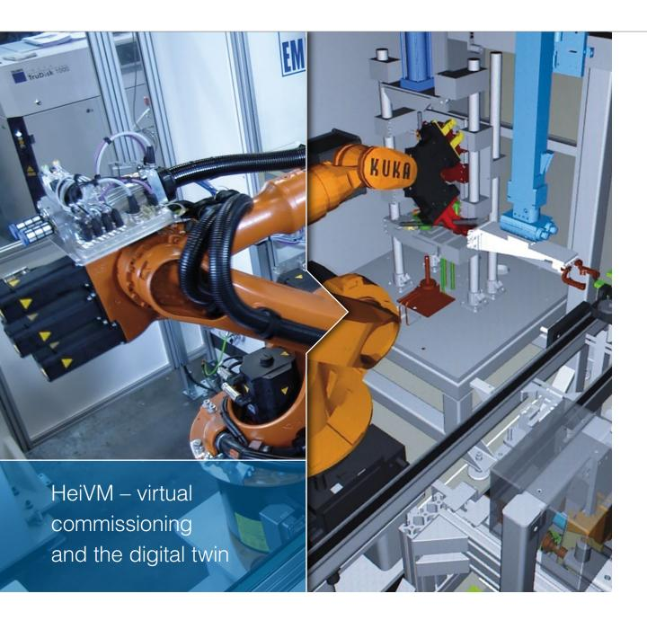
During plant design, software-based support of engineering processes using virtual models of machines, plants, robot applications, and material flows is a key driver of productivity. With the aid of the virtual twin, engineers are able to test the functionality and time response of automation concepts and optimize process sequences before implementation.
